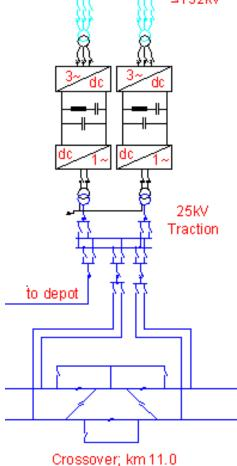
Standard transformer traction power substation in Vconnection (low cost)
